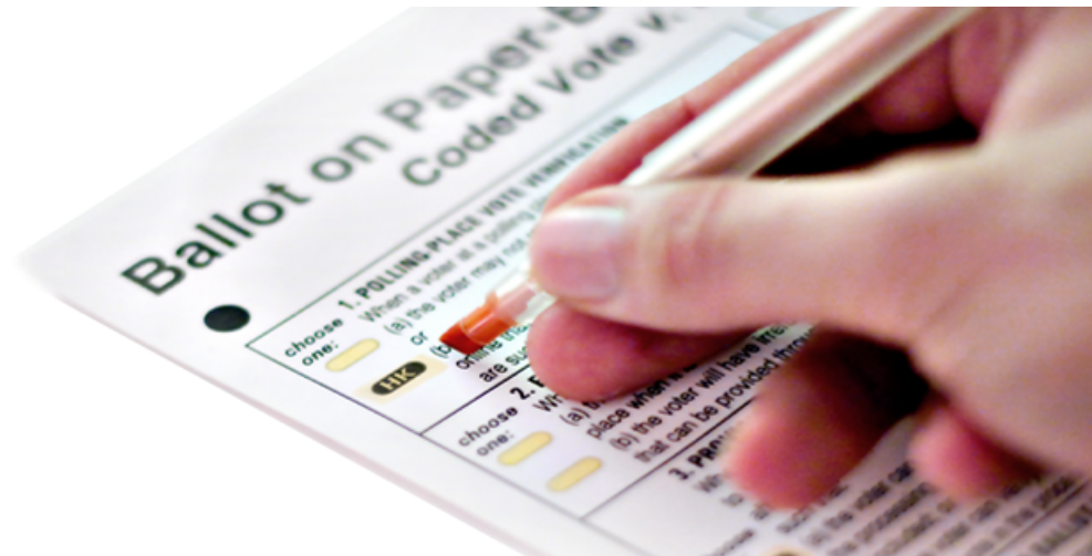
Figure 2.3: Example Scantegrity ballot. Special verification codes are printed onto the ballot with invisible ink. Voters reveal the codes by marking the bubbles with a special pen, and verify these codes against the public bulletin board after the election. Standard PCOS scanners will read the marked Scantegrity ballot. (Image from [81])
